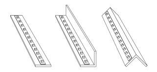
For a seamless glow and to avoid bright light spots, move the LED tape light strip further from adjacent walls.
